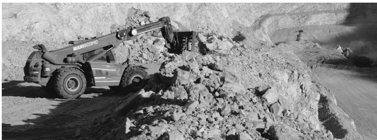
Figure 2 Telescoping handler commencing rock fall test
